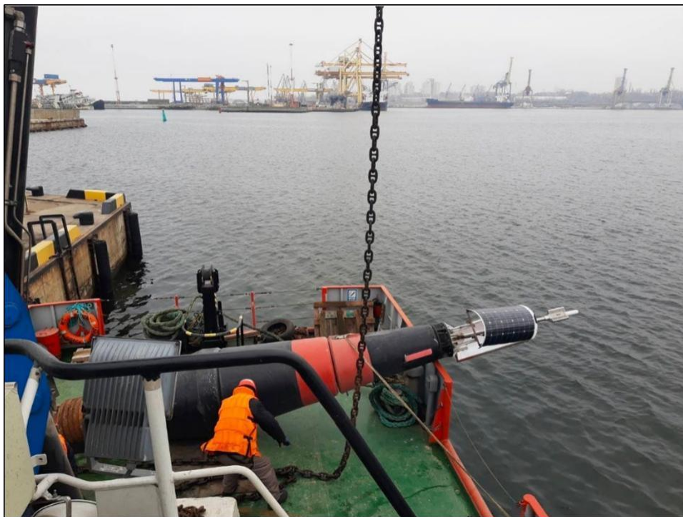
Figure 2-2. Black Sea Deployment of Ukrainian Bouy with Acoustic Sensor
