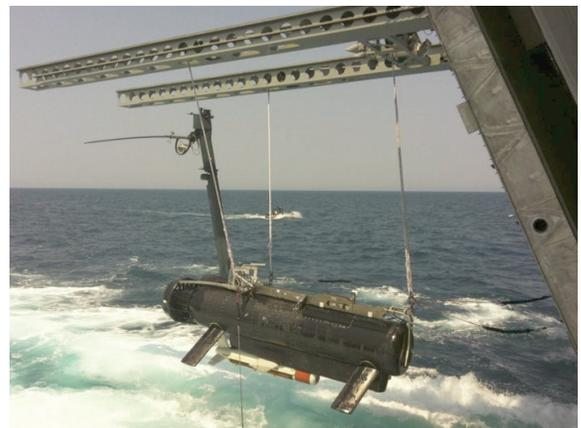
The RMS program has not yet demonstrated that the system can meet its detection and classification requirements against moored and bottom mines spanning the portion of the shallow water regime not covered by the Airborne Laser Mine Detection System (ALMDS). The program anticipates that the AN/AQS-20B sensor will permit the system to cover the portion of the water column below that covered by the ALMDS. The new sensor will be tested in FY15.
