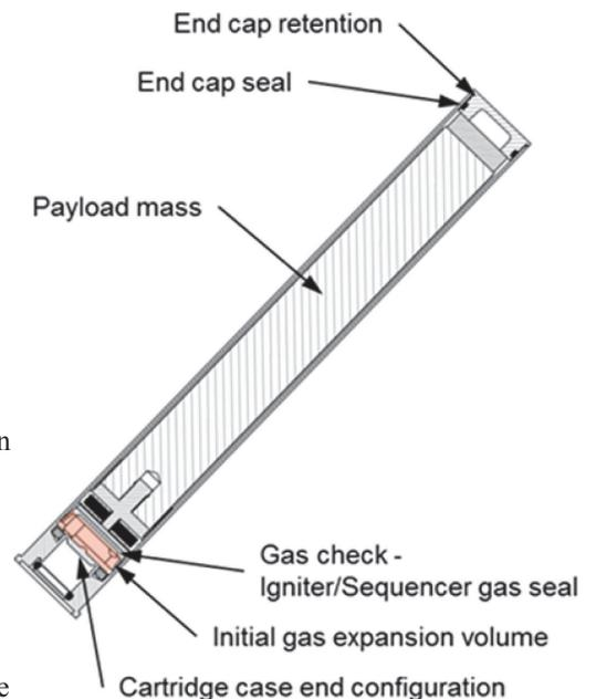
a desired ejection velocity is obtained and parameters that affect it are identified, a common impulse cartridge for all Services will be more easily achievable, thereby reducing support costs. In the next phase, NSWC-Crane will conduct a flight test to determine how tailored flares improve effectiveness. Methods to adjust ejection velocity will be used to enhance effectiveness of current expendables.
