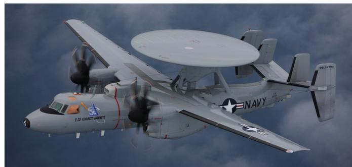
support increased aircraft weight; replacement of the radar system, the communications suite, and the mission computer; and the incorporation of an all-glass cockpit, which permits the co-pilot to act as a tactical fourth operator in support of the system operators in the rear of the aircraft.
