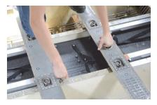
better durability and less installed weight. Locating the armor under the cabin floor panels greatly reduces the wear and increases its lifespan. The designers also developed an installation and removal system that is lightweight,
