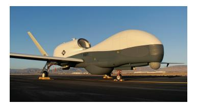
electro-optical/infrared sensor provides full motion video and still imagery of surface targets. An Electronic Support Measures system detects, identifies, and geo-locates radar threat signals. An Automatic Identification System (AIS) receiver permits the detection, identification, geo-location, and tracking of cooperative vessels equipped with AIS transponders.
