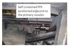
requiring an external power source. The FPS will incorporate
