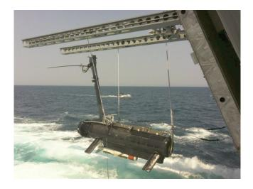
and volume (in the water column) mine-like-contacts. The sensor utilizes a port and starboard Side-Looking Sonar and a Gap Filler Sonar for detection of bottom and tethered volume mines. A Volume Search Sonar (VSS) and a Forward-Looking Sonar are utilized for all mine type detection. An Electro-Optic Identification Device can replace the VSS for missions requiring (mine versus non-mine) identification of shallow-water bottom mine-like-contacts via high-resolution imaging.
