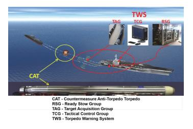
processing equipment. Data from the array and the ship's radar system are processed into contact tracks and alerts to be forwarded to the Tactical Control Group. The array will eventually be capable of both passive and active sonar operations.
