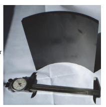
additional weight reduction over current solutions. The armor consists of a continuous fiber-reinforced glass-CMC strike face, bonded directly (no adhesive) to a monolithic ceramic, which is in turn directly bonded to a second layer of fiber-reinforced glass-CMC, backed by a final layer of highly cross-linked polyethylene fiber.
