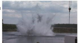
the middle of the water column, and at keel depth for floating structures. In FY13, the test results were analyzed to better understand the test pond bottom characteristics, explosion bubble migration, and shock loading. This project effectively leverages a joint U.S./German investment of nearly \$20 Million and provides data to increase the fidelity of models and the accuracy of survivability assessments, as well as addresses fleet urgent operational needs.
