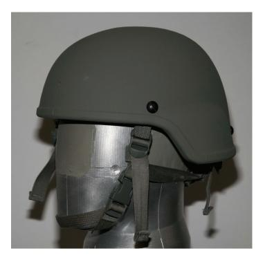
using ultra-high-molecular-weight polyethylene fibers. Unlike aramid composites, the ultra-high-molecular-weight polyethylene ballistic material absorbs ballistic impact and dissipates energy via extensive plastic strains. This results in more resistance to penetration but it also results in large permanent helmet shell deformations and larger damaged areas following impact for a wide range of ballistic threats.
