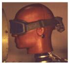
testing using a Facial and Ocular Countermeasure for Safety head form. The primary test objectives were to assess the level of blast protection that goggles and spectacles provide Soldiers during blast events, to quantify pressure levels seen in the ocular region during blast events, and to indicate any design features that
