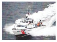
Coast Guard 41-foot utility boat, which is being taken out of service. The Coast Guard has made a number of these boats available to the Navy as targets representing fast-attack craft. JLF-Sea funded NSWC, Dahlgren, to develop a target geometry model for the boat and to
