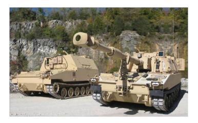
common chassis with the SPH. The ammunition carriers are designed to carry 12,000 pounds of ammunition in various configurations and a crew of 4 Soldiers.
