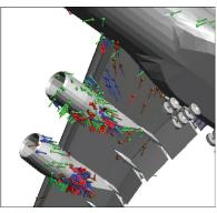
MANPADS engagement M&S facilities modeled specific MANPADS threats. A statistical comparison of the results and an analysis to validate MANPADS hit point prediction simulations was conducted. In FY11, the team will complete correlation of M&S hit point prediction test results with available live fire data, and develop a standardized methodology for hit point prediction simulations, improving MANPADS vulnerability analyses.
