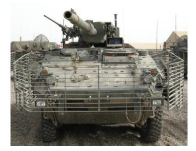
provided by add-on slat armor (high hard steel arranged in a spaced array).
