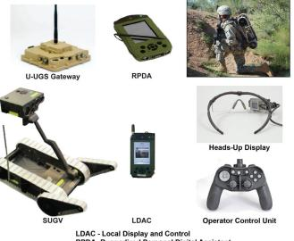
LDAC - Local Display and Control RPDA- Ruggedized Personal Digital Assistant SUGV - Small Unmanned Ground Vehicles U-UGS - Urban-Unattended Ground Sensors
